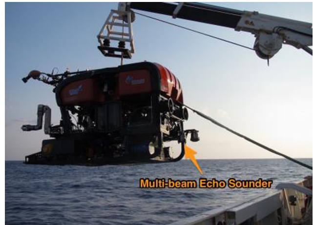
Fig. 3 Multi-beam Echo Sounder on the stern of the Hemire
