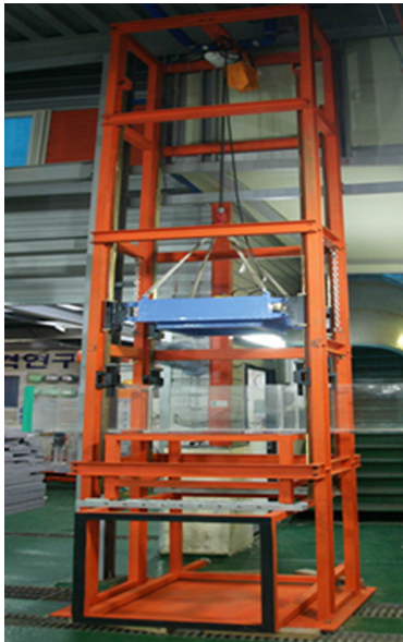
Fig. 1 Wet drop test rig
