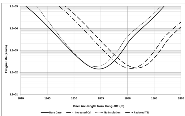
Fig. 13 Fatigue sensitivity result with respect to design parameters at touch-down zone
