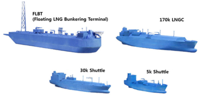
Fig. 2 Models for wind tunnel tests
