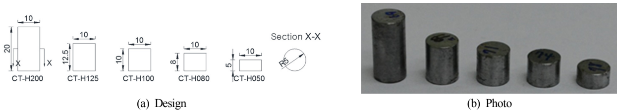
Fig. 5 Compression specimens (Choung et al., 2015a)
