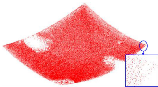
(b) Measured points using 3D laser scanner (21,918 points)
