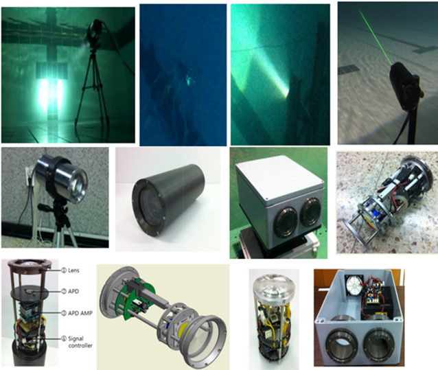
Fig. 6 Optical Communication Modems of Korea Maritime University
