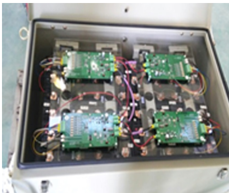
Fig. 4 View of energy-conservation unit (battery) set up in electric ship
