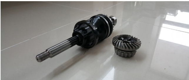
Fig. 7 View of bevel reduction gear & propeller shaft in lower unit
